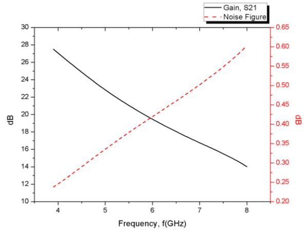
Figure 8: Simulated gain and noise figure of wideband LNA
