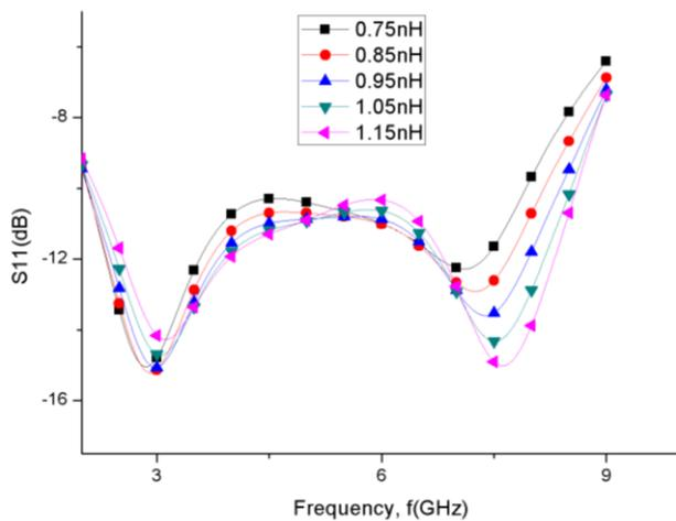
Figure 3: Analysis of input impedance network by varying inductor,  $L_s$
