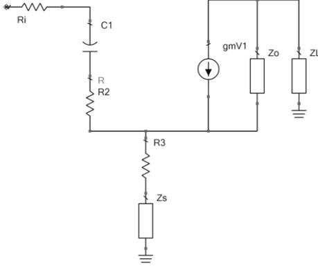
Figure 2: Common source amplifier with source degeneration.
