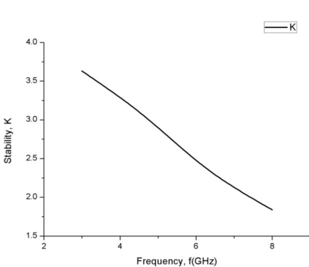
Figure 6: Simulated stability of wideband LNA
