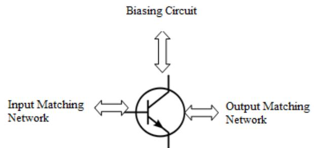
Figure 1: Basic block diagram of LNA.
