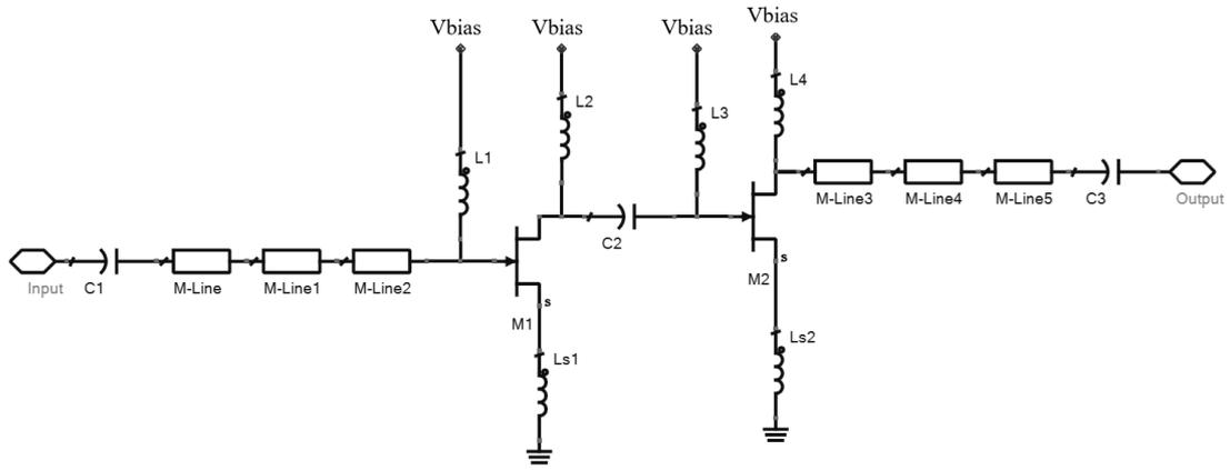
Figure 5: The schematic diagram of low noise amplifier with multi-section quarter wave transformer
