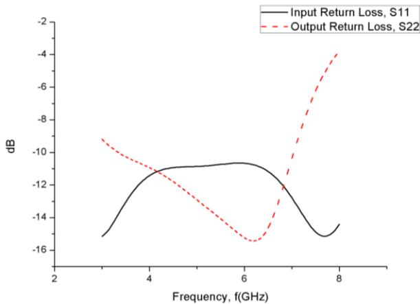
Figure 7: Simulated input and output return loss of wideband LNA
