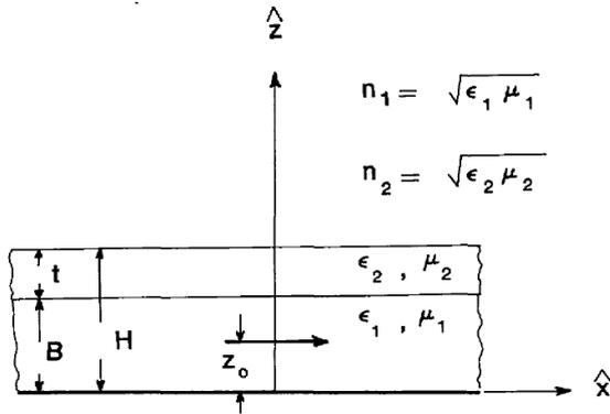
Figure 6: Superstrate-Substrate Geometry [16].
