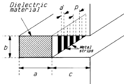
Figure 10: Metal Strip Loaded Dielectric Waveguide [18].
