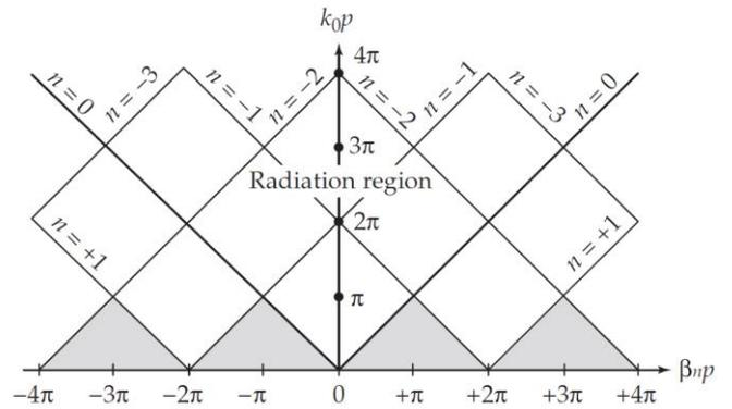
Figure 16: Brillouin Dispersion Diagram for a periodic Structure Showing Radiation (Fast-Wave) Region And Bound Modes (Shaded Regions) For Slow Wave Space Harmonics [23][26].
