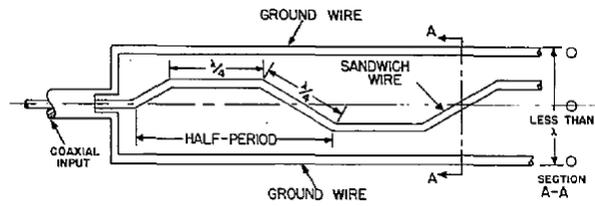
Figure 3: Sandwich Wire Antenna [13].
