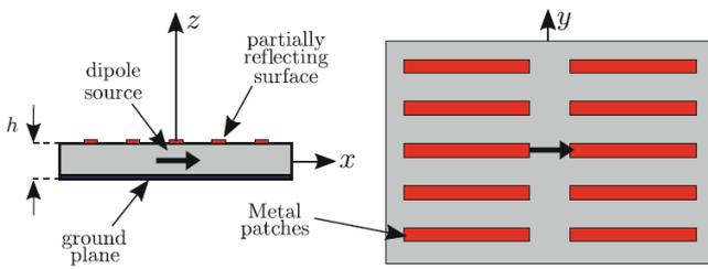
Figure 24: Construction of a Partially Reflecting Surface Using Metal Patches [35]
