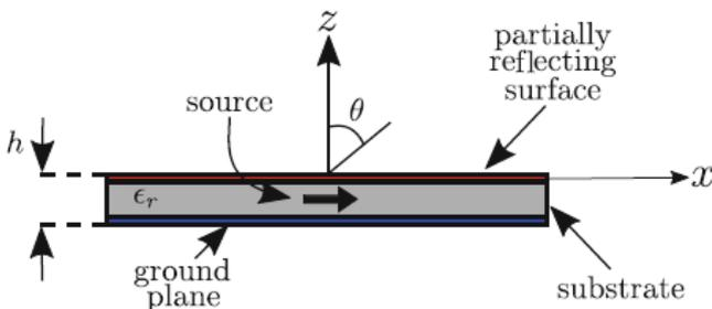
Figure 23: Substrate/superstrate structure of a two-dimensional leaky-wave antenna [35][36]
