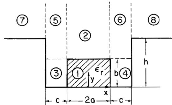
Figure 5: Cross Section Of The Dielectric Waveguide Used [15].
