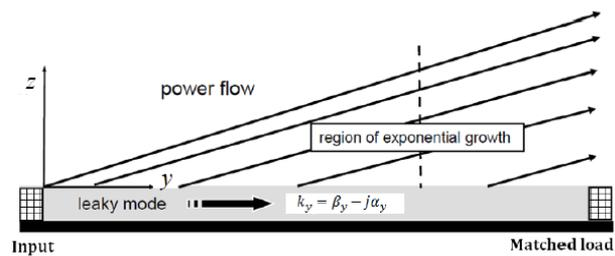
Figure 13: Scheme of The Near Field Created By a Forward Radiating Lw in a Quasi-Uniform One Dimensional LWAs [24][25]
