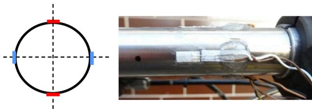
Figure 2: Detail and placement of strain gauges and detail
