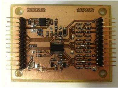
Figure 4: Electronic board with A/D converter for measuring
