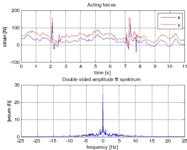
Figure 12: Hitting measurement
