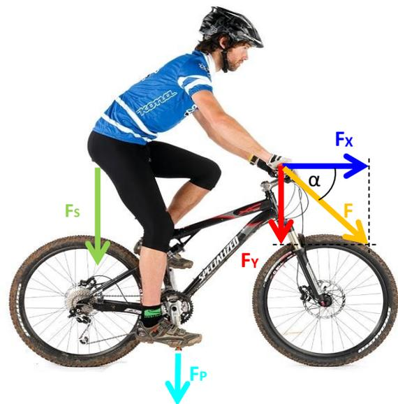
Figure 1: Forces between human and the vehicle
