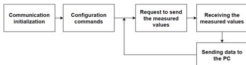
Figure 6: Communication block scheme
