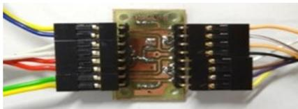
Figure 5: External board with Wheatstone bridges' resistors
