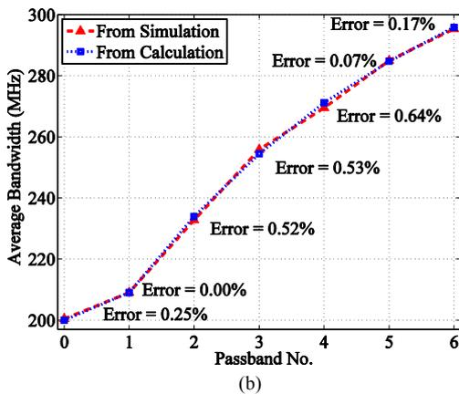
Figure 5: (a) The average bandwidth evaluated from Equation (5), and (b) The error between the simulation and calculation for the average bandwidth with  $t_{d,dev} = 2.50$  ns.
