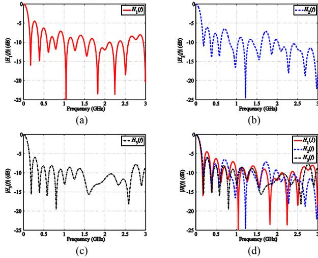
Figure 1: Magnitude response of the complex envelope of the multimode fiber modeled by (2) with  $N_{mode} = 100$ ,  $t_{d,avg} = 5 \mu s$ , and  $t_{d,dev} = 2.50$  ns. Three responses correspond to three different sets of delays
