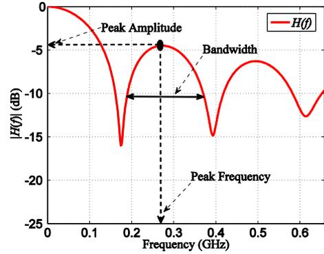
Figure 2: Three important passband parameters to be studied
