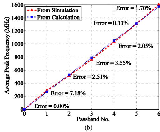
Figure 4: (a) The average peak frequency evaluated from Equation (4), and (b) The error between the simulation and calculation for the average peak frequency with  $t_{d,dev} = 2.50$  ns.
