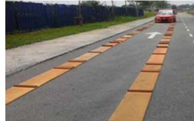
Figure 4: Running Test Car on Artificial Road Surface
