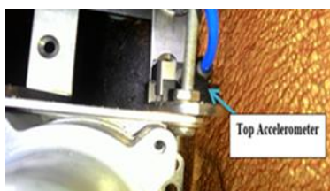
Figure 2: Accelerometer Sensor Installation for Vertical Body Acceleration
