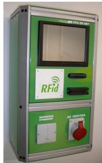
Figure 1: Charging stand developed at VSB-TU Ostrava. The big display allows to implement additional features as web browser using etc.
