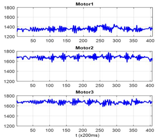
Figure 1: PWM signals of the three main blade servos
