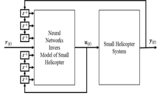
Figure 5: Neural Networks Direct Inverse Control (NN-DIC)
