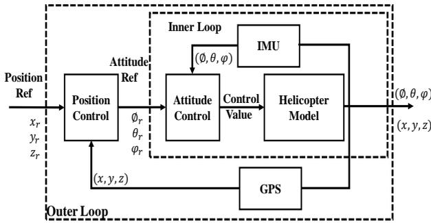
Figure 4: The block diagram of a general control system of a helicopter
