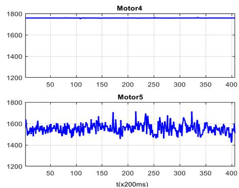
Figure 2: PWM signals of the BLDC and the tail blade servo
