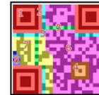
Figure 3: The structure of QR code version 2
