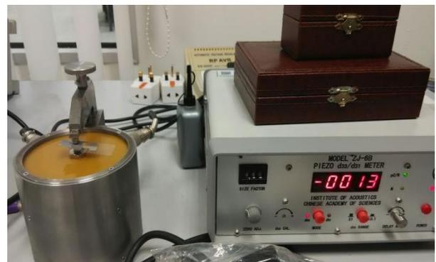
Figure 7: Direct measurement of piezoelectric coefficient,  $d_{33}$ .
