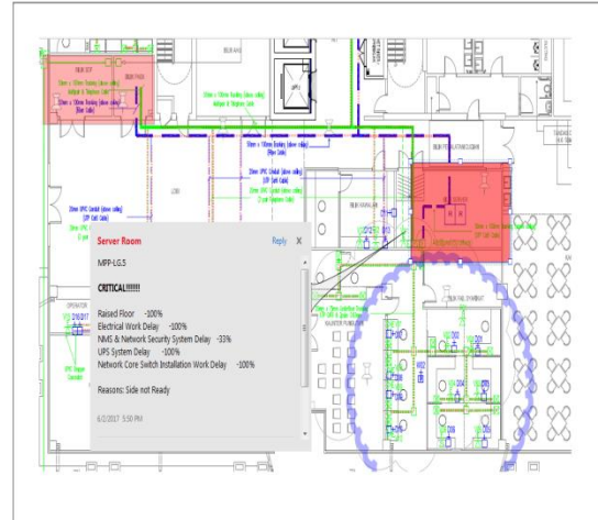
Figure 7: Drawing shows Server Room in red (critical stage) and percentage of work report
