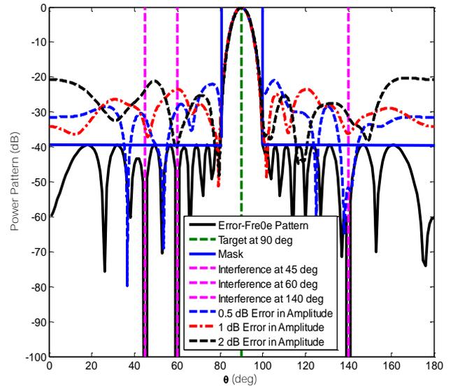
Figure 4: Effect of random errors in the array amplitude on the adaptive nulling for  $N=20$  elements, and three nulls at 45, 60, and 140 deg.
