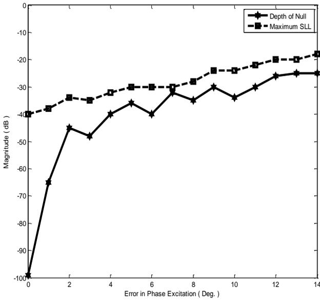
Figure 7: The depth of the null and the peak sidelobe level versus random errors in phase excitation.
