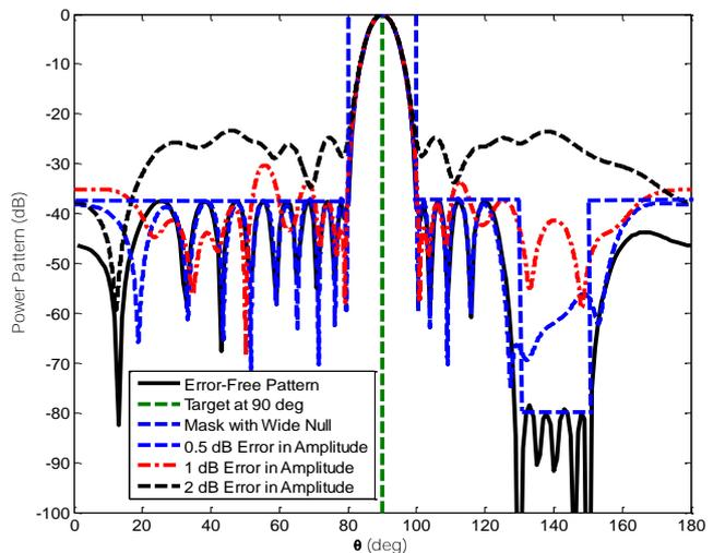
Figure 6: Effect of random errors in the array amplitude on the adaptive nulling for  $N=20$  elements, and wide null around 140 deg.
