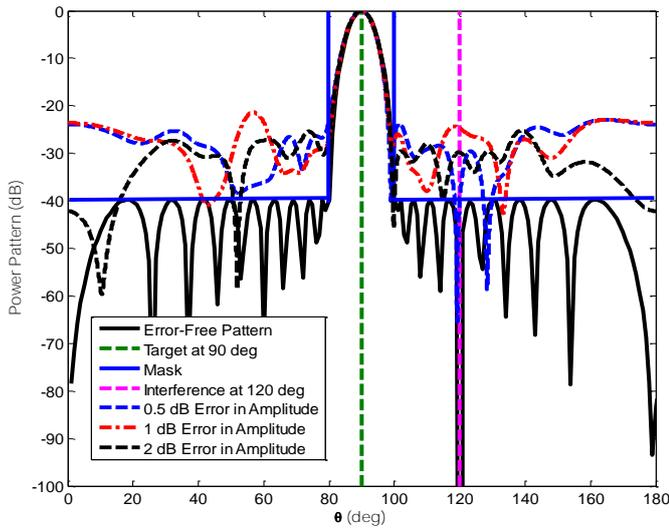
Figure 2: Effect of random amplitude errors on the adaptive nulling for  $N=20$  elements, and a single null at 120 deg.
