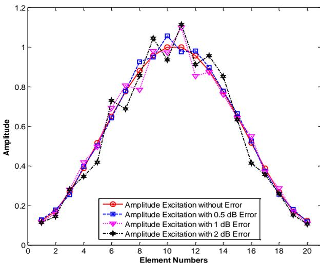
Figure 9: The arrays weights for various levels of error in the amplitude.
