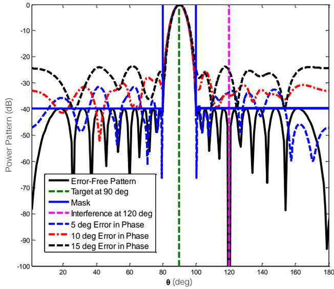
Figure 1: Effect of random phase errors on the adaptive nulling for  $N=20$  elements, and a single null at 120 deg.
