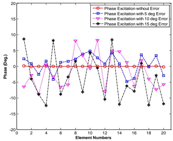
Figure 10: The phases of the array weights for various levels of error in the phase
