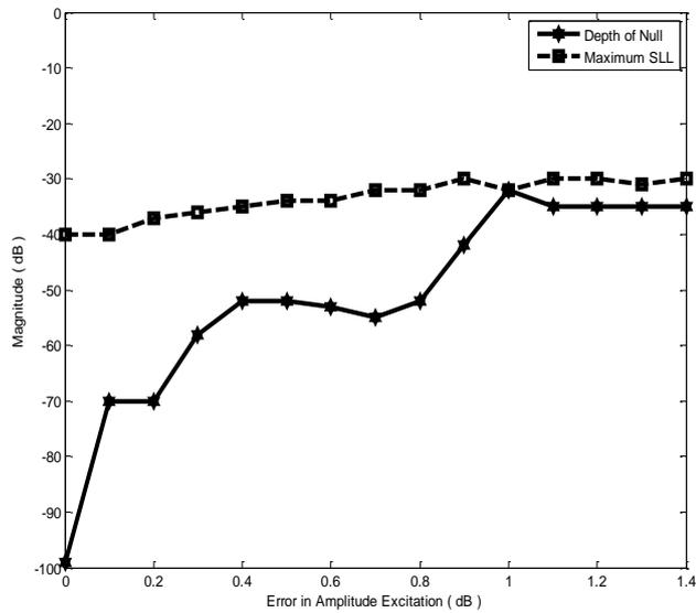
Figure 8: The variation of the null depth and the peak sidelobe level versus random errors in amplitude weights.
