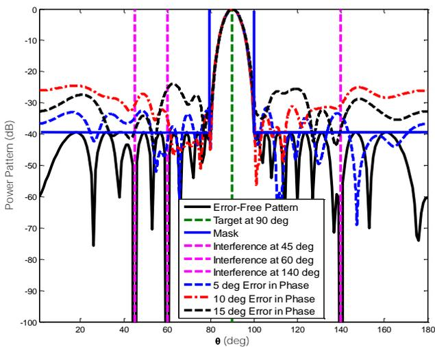
Figure 3: Effect of random errors in the array phases on the adaptive nulling for  $N=20$  elements, and three nulls at 45, 60, and 140 deg.
