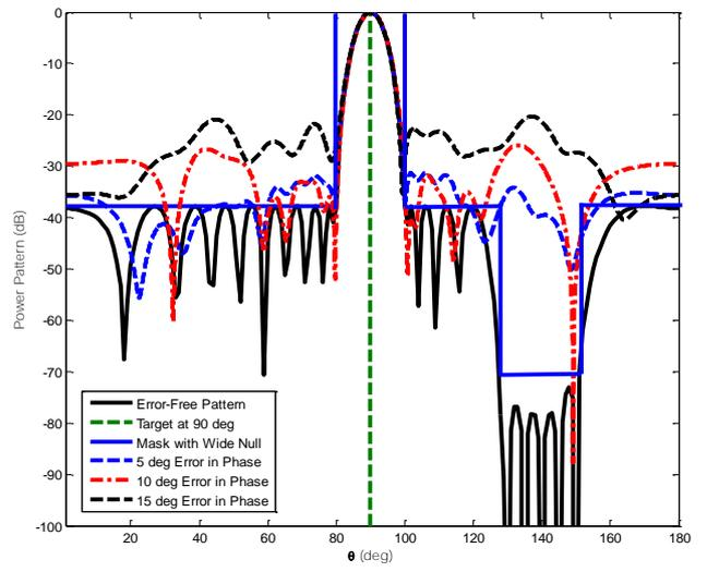
Figure 5: Effect of random errors in the array phases on the adaptive nulling for  $N=20$  elements, and wide null around 140 deg.
