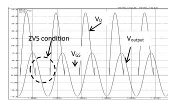
Figure 8 Simulated  $V_{GS}$ ,  $V_{DS}$  and  $V_{output}$  of the Class E ZVS inverter after tuning process
