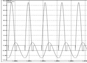
Figure 7. Simulated  $V_{\text{GS}}$  ,  $V_{\text{DS}}$  and  $V_{\text{output}}$  of the Class E ZVS inverte
