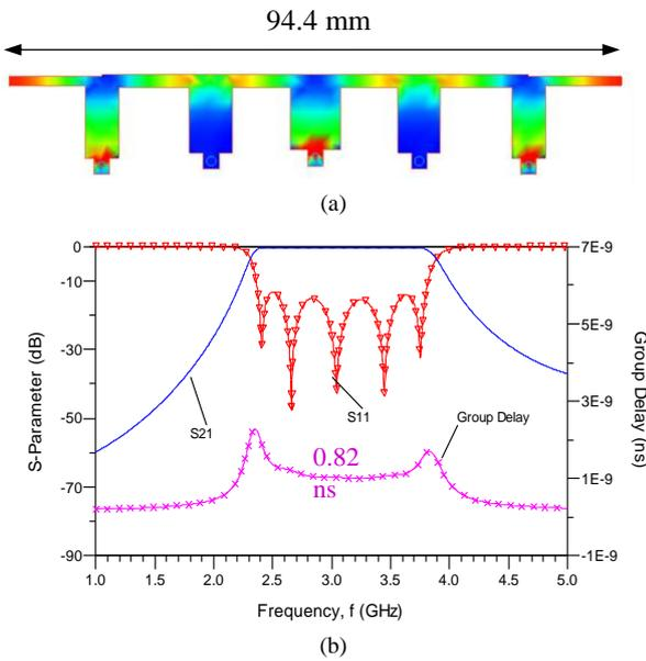
Figure 1: Simulation response (a) Current flow visualization of band-pass filter short circuit stub at 3.1 GHz and (b) Simulated response of band-pass filter short circuit stub with group delay.
