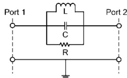
Figure 3: Equivalent circuit of DMS structure
