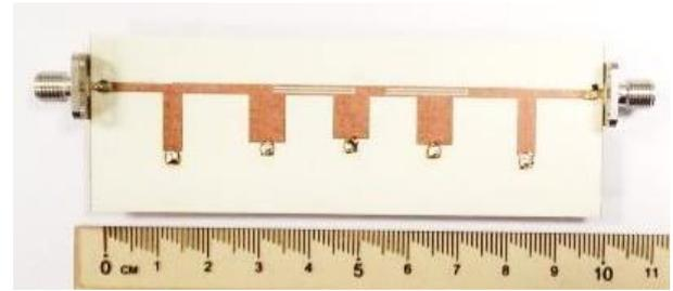
Figure 6: Fabricated of dual-band bandpass filter
