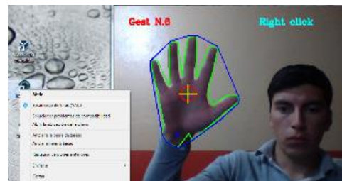
Figure 7: a) Contour hand, b) Convex hull, c) Center of mass location and d) Defects convexity
