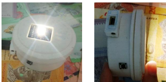
Figure 10: The 3D printed casing for the banknote recognition device.
