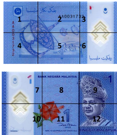
Figure 1: RM 1 banknote sample with 12 points used to collect data for R, G, and B values.
