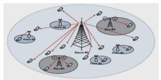
Figure 2: RSRP based Cell Association of a Three-Tier HetNet [12].
