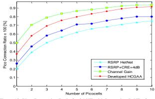
Figure 12: Pico Connection Ratio for 25 UE with Increasing PeNBs for Configuration 1
