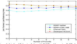
Figure 8: Jain Load Balancing Index with 25 UE and Increasing PeNBs for Configuration 1
