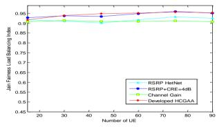
Figure 7: Jain Load Balancing Index with 4 PeNBs and Increasing UE for Configuration 4b
