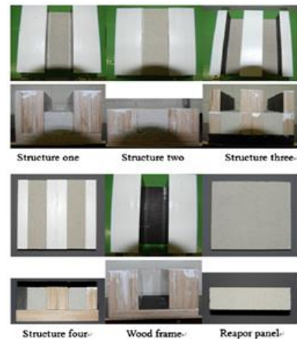
Figure 1: Wooden rectangular periodic groove structure with porous material [4]
