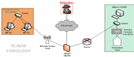
Figure 1: Testbed Environment of Secured SCADA Topology Using IDS-Mikrotik
