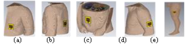
Figure 3: Different antenna placement on Hugo voxel model (human body): (a) chest; (b) back; (c) abdomen; (d) arm; (e) thigh
