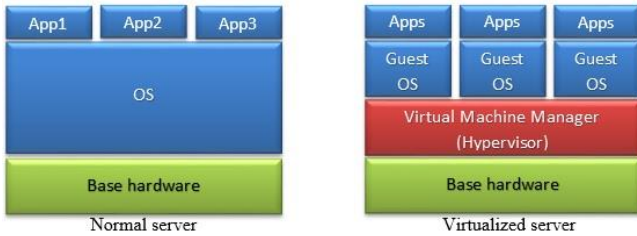
Figure 1: Virtualized Server Architecture
