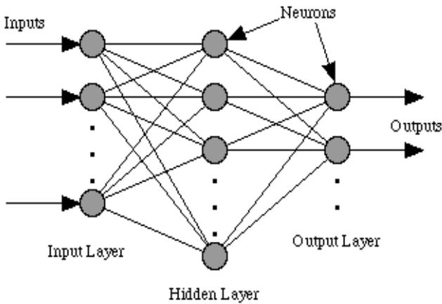
Figure 3: The MLP feedforward neural network architecture
