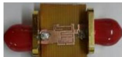
Figure 1(b): Fabricated structure of proposed filter
