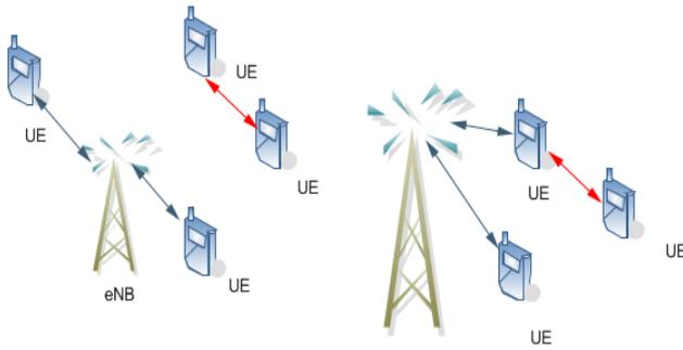
Figure 3: Device to Device Communication
