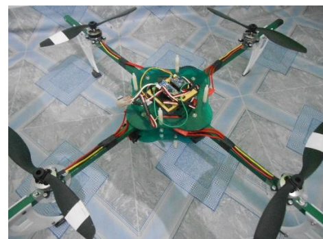
Figure 9: Implementation of the quadrotor mechanical design
