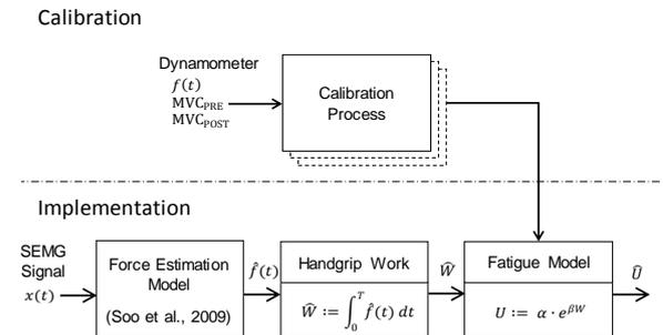
Figure 2: Overview of the proposed method for quantifying the degree of muscle fatigue using SEMG signal.
