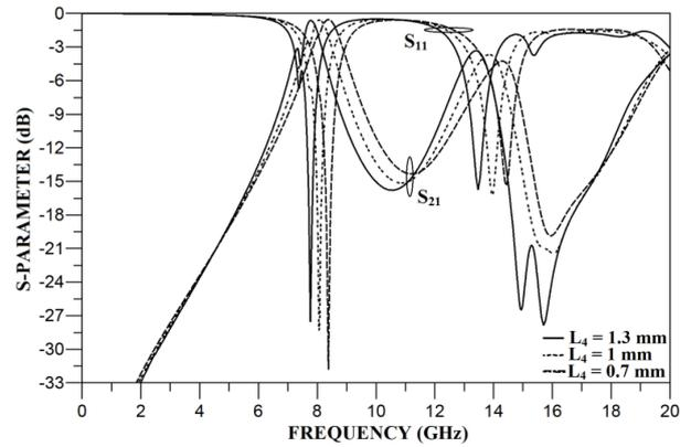
Figure 7: Frequency response of cascaded open loop triangular ring resonator with varied stub length  $L_4$ .
