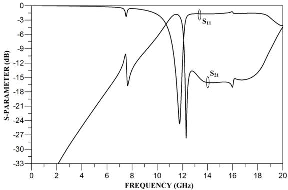
Figure 12: Frequency response of proposed filter.
