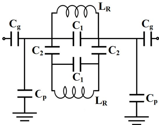
Figure 6: Equivalent circuit of cascaded open loop triangular ring resonator loaded with stub.
