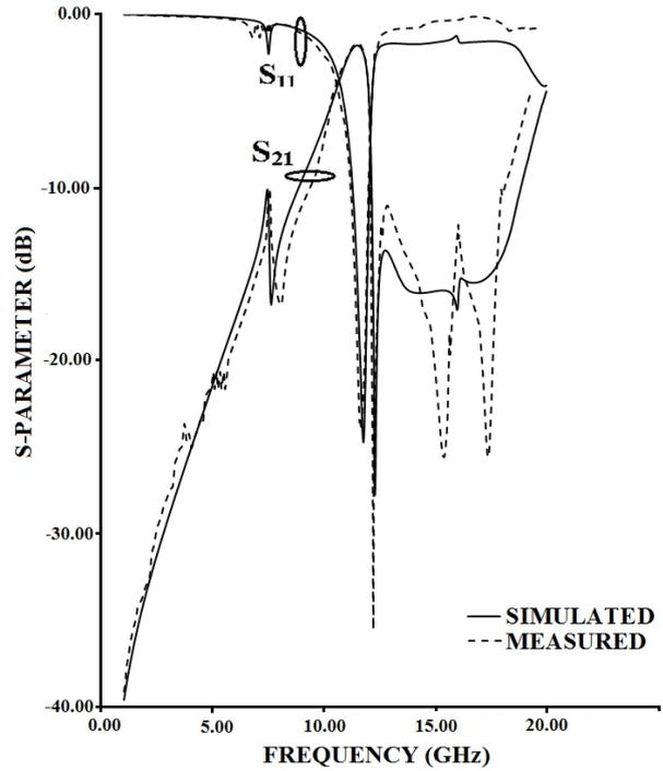
Figure 14: Simulated and measured Frequency response of the proposed filter.
