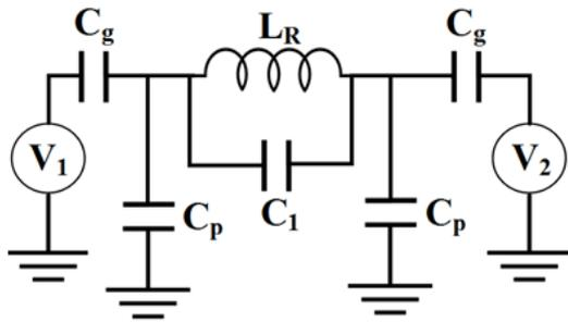
Figure 3: Structure of open loop triangular ring resonator coupled in series with transmission line.
