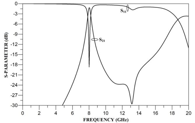
Figure 4: Frequency response of open loop triangular ring resonator coupled in series with transmission line.
