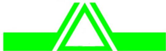
Figure 1: Configuration of the conventional triangular dual-mode filter
