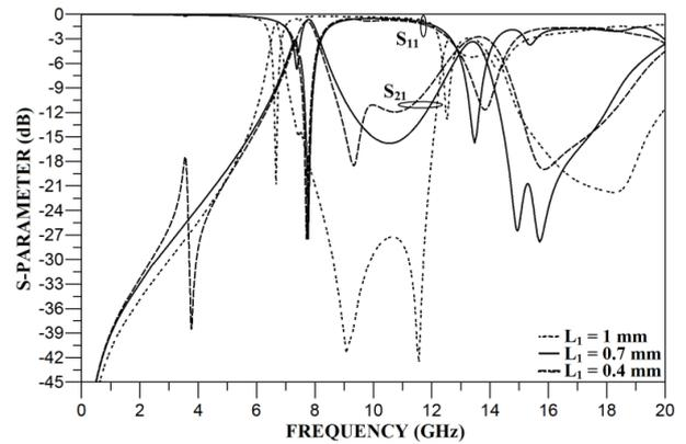
Figure 8: Frequency response of cascaded open loop triangular ring resonator with varied length  $L_1$
