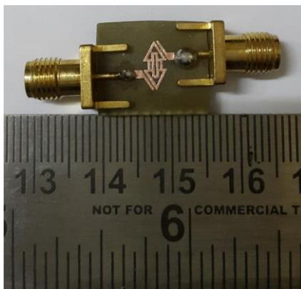
Figure 13: Photograph of the fabricated proposed Filter.
