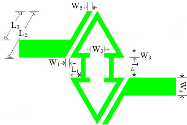
Figure 5: Structure of cascaded open loop triangular ring resonator loaded with stub.
