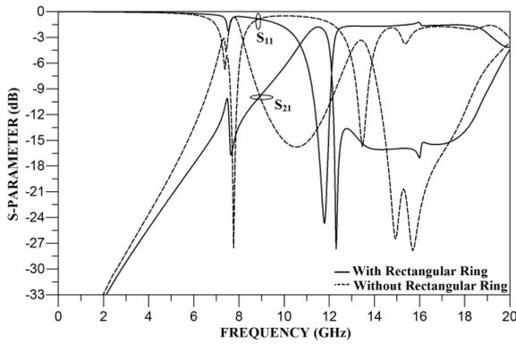
Figure 11: Comparative frequency response of proposed filter with and without rectangular ring.
