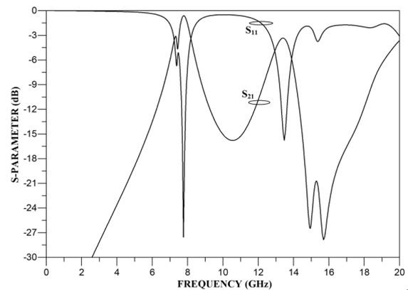
Figure 9: Frequency response of cascaded open loop triangular ring resonator loaded with stub.
