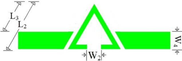
Figure 2: Structure of open loop triangular ring resonator coupled in series with transmission line.
