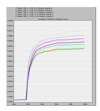
Figure 6: End-to-end delay of all VOIP responders
