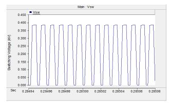
Figure 7: Simulated waveforms of switch  $S_1$  ( $V_{S1,max} = 383V$ ).
