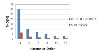
Figure 5: Harmonic content of input current compared with IEC 6100-3-2 Class C.
