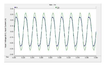
Figure 6: Simulated waveforms of input voltage ( $V_{in} = 230$  Vrms) and input current ( $i_{in} = 0.24$  Arms)
