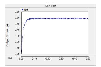
Figure 10: Simulated waveforms of output current ( $I_0 = 0.59$ A)
