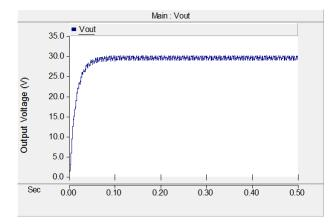
Figure 11: Simulated waveforms of output voltage (Vo = 29V).
