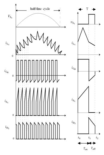
Figure 3: Operating waveforms of the proposed SEPIC-flyback converter.
