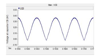
Figure 8: Simulated waveforms of capacitor  $C_{\mathbf{B}}$  voltage ( $V_{CB,max}$ = 365 V).
