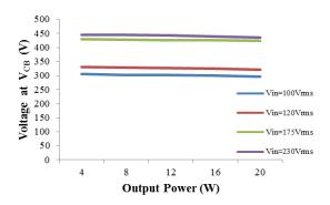
Figure 9: Capacitor  $C_{\rm B}$  voltage over load variation.
