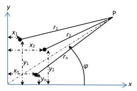
Figure 1: Schematic diagram of dipole placement
