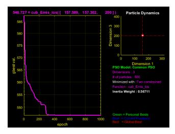
Figure 2: Convergence curve of the PSO for emission dispatch considering transmission loss
