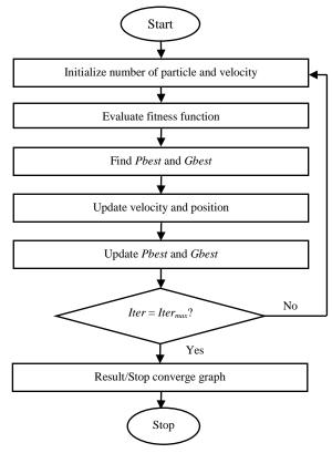
Figure 1: Flow chart of Particle Swarm Optimization
