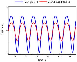
Figure 5: Tracking motion for Lead-plus-PI and 2-DOF Lead-plus-PI with frequency 0.5 Hz and amplitude 1.0 mm
