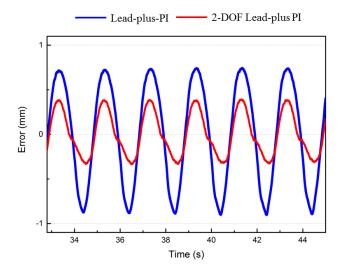
Figure 4: Tracking motion for Lead-plus-PI and 2-DOF Lead-plus-PI with frequency 0.5 Hz and amplitude 0.5 mm
