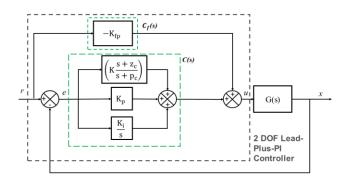
Figure 2: Block diagram of 2-DOF Lead-plus-PI controller
