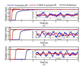
Figure 3: Step response to (a) 6 mm (b) 5 mm and (c) 4 mm jump height
