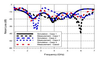
Figure 7 : Return Loss for all cases along H-plane bending
