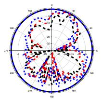
(b) Azimuth radiation pattern of E-plane at 5.2 GHz
