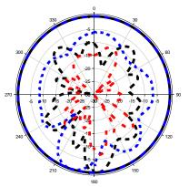
(c) Azimuth radiation pattern of H-plane at 2.4 GHz
