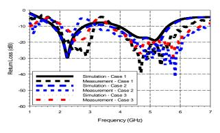
Figure 6 : Return Loss for all cases along E-plane bending
