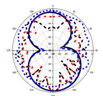
(c) Elevation radiation pattern of H-plane at 2.4 GHz
