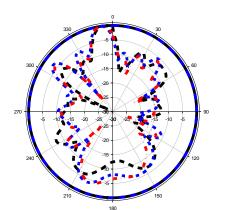
(a) Azimuth radiation pattern of E-plane at 2.4 GHz
