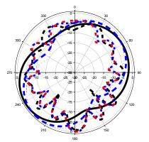
(a) Elevation radiation pattern of E-plane at 2.4 GHz
