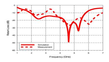
Figure 2 Simulated and measured return loss comparison on flat antenna condition
