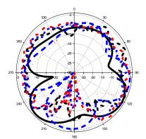
(b) Elevation radiation pattern of E-plane at 5.2 GHz
