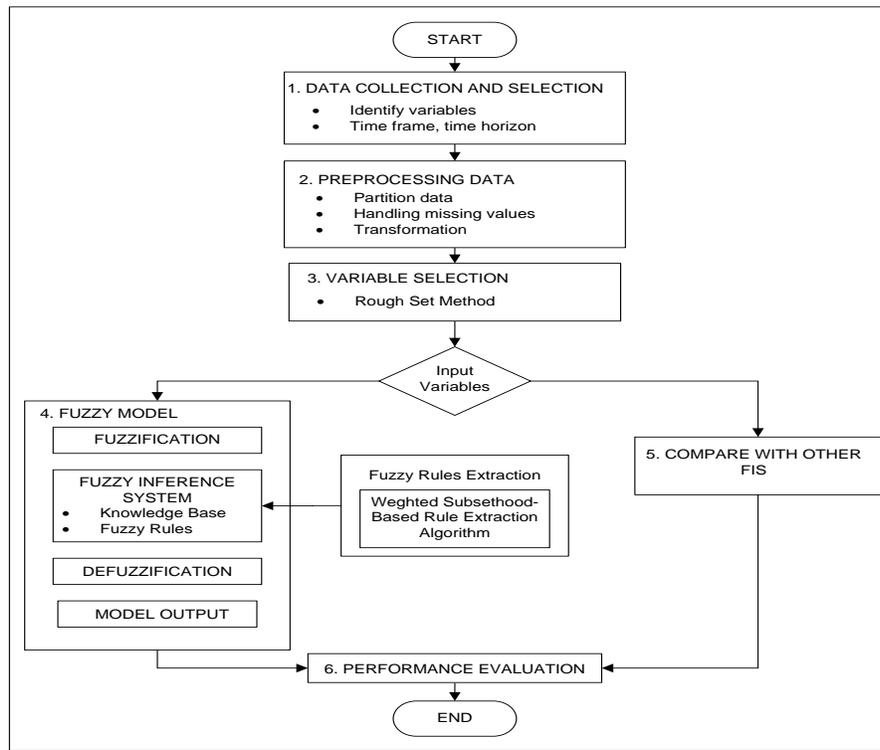
Figure 1: Proposed MFRBS-WSBA for electricity load demand forecasting
