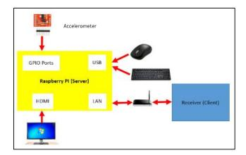
Figure 3: The block diagram (hardware) of the system
