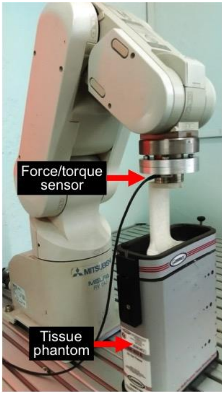
Figure 4: Data acquisition setup for tissue phantom
