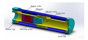
Figure 10: Cross-sectional view of linear actuator.
