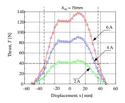
Figure 8: Performance current characteristic.
