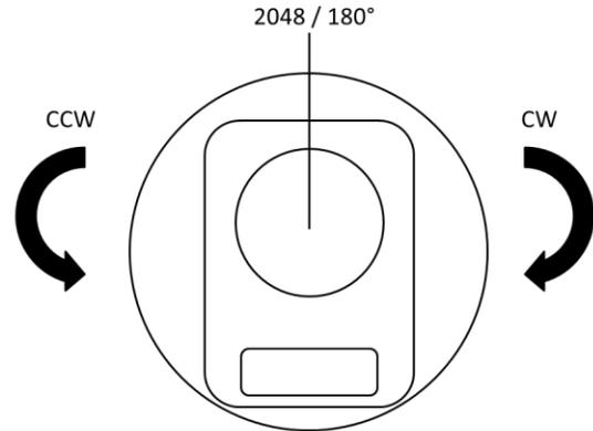
Figure 3: Illustration of Goal position in Dyanamixel motor.
