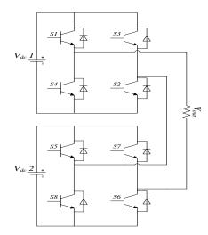
Figure 4: Cascaded H-bridge (CHB) multilevel inverter
