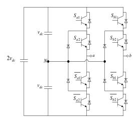
Figure 2: Neutral point clamped multilevel inverter
