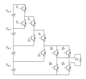
Figure 11: H-Bridge and two-level power modules (HBTPM)-based multilevel inverter
