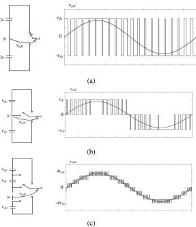
Figure 1: Basic concepts of inverters (a) Two-level (b) Three-level (c) Nine-level
