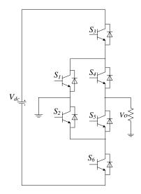
Figure 5: Active NPC multilevel inverter
