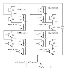
Figure 9: Modular multilevel converter
