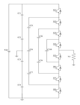
Figure 3: Flying capacitor multilevel inverter
