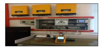
Figure 3: The setup connection of Fluke 43B for measurement and recording data.
