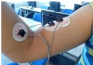
Figure 2: Surface EMG electrode's placement at the right biceps.
