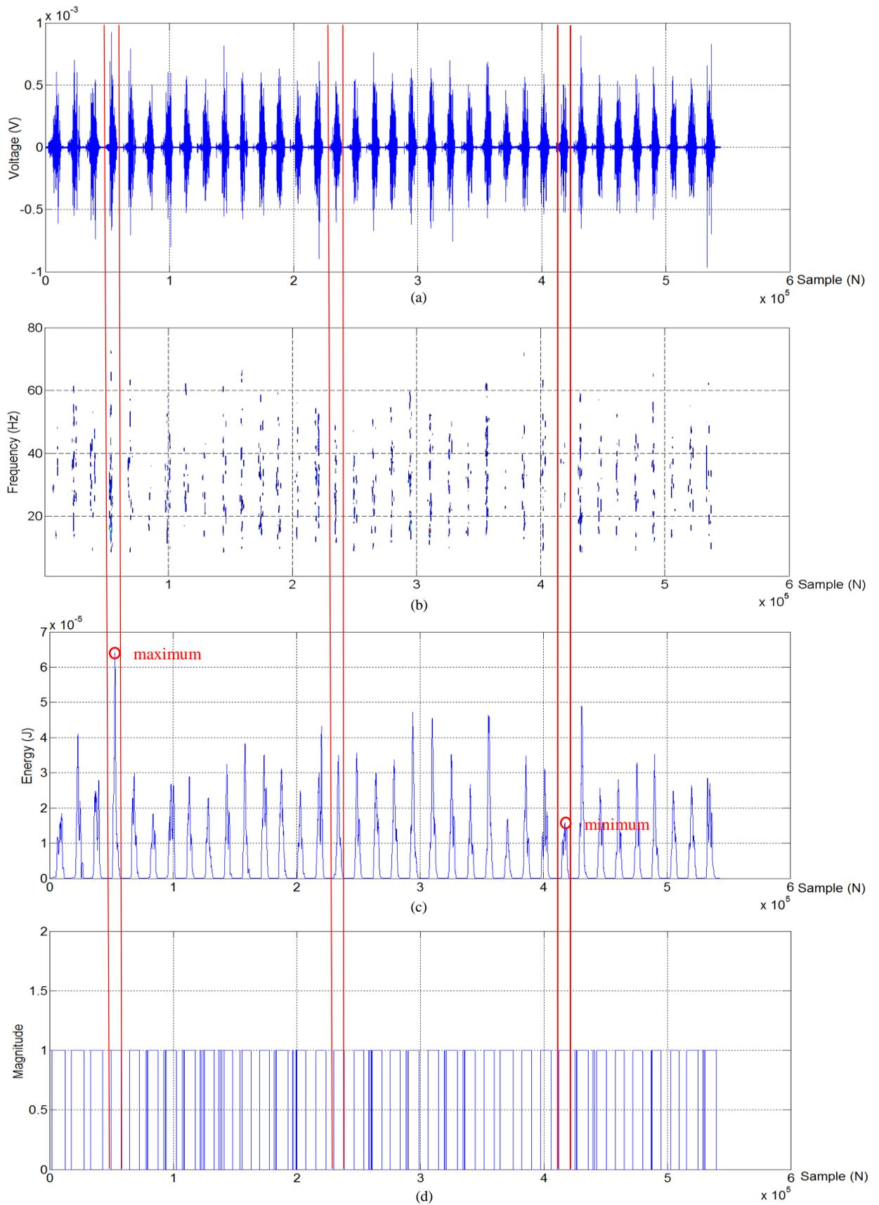
Figure 6: (a) The raw sEMG signal obtained from biceps brachii during manual lifting. (b) The time-frequency representation of the overall signal. (c) The instantaneous energy for each muscle contraction. (d) Activation intervals for each muscle contraction obtained using the threshold calculation.
