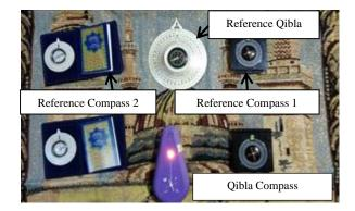
Figure 7: Mosque Qibla direction, reference compass 1 and 2, and Qibla compass placed for validation at the mosque
