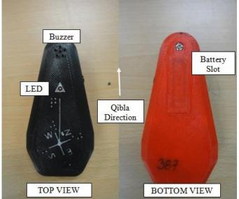
Figure 6: Qibla compass final design
