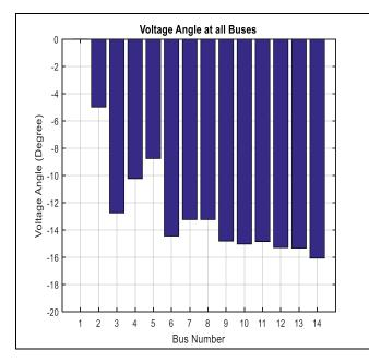
Figure 4: Voltage angle values at all buses
