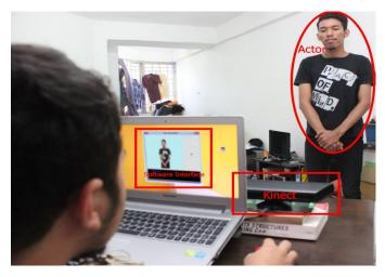
Figure 1: Examples of possible usage of Kinect for sign language interpreter
