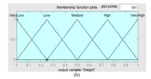
Figure 1: Fuzzy Logic: Triangular function of input (RSSI) (a) and output (weight) (b)
