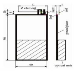
Figure 7: Metamaterials inspired inverted F antenna (MIIFA) [28].
