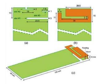
Figure 1: a) Front view of PCB, (b) front view of the antenna, and (c) 3D view of the antenna. PCB is 100 mmX40 mm. Height of the PIFA is 6 mm. [12].
