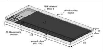
Figure 3: Monopole antenna for octaband mobile application [17].
