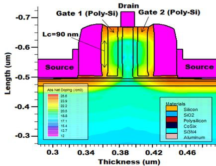
Figure 3: Contour mode of Vertical Double Gate NMOS device
