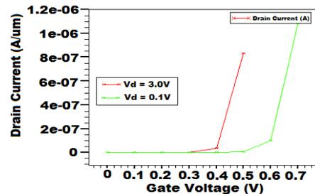
Figure 6: Graph  $I_D$ - Ramp  $V_G$  for Vertical Double Gate NMOS Device
