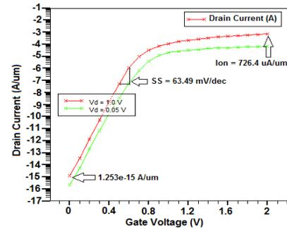
Figure 5: Graph of subthreshold drain current ( $I_D$ ) vs. gate voltage ( $V_G$ )
