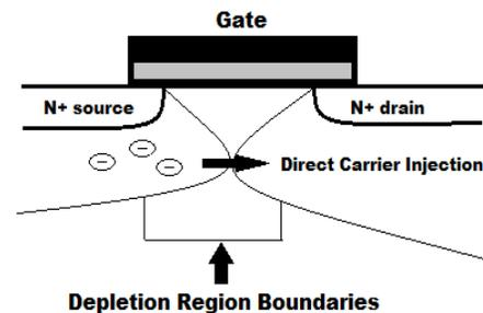
Figure 1: Direct carrier injection
