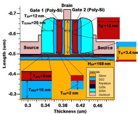
Figure 2: Vertical Double Gate NMOS Structure
