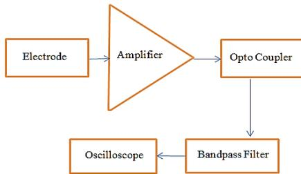
Figure 9: Function block of the KL-75001 ECG Module
