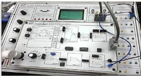
Figure 3: KL-75001 Electrocardiogram ECG Module and KL-72001 Biomedical Measurement System Module board
