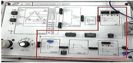
Figure 8: Filtering segment on the KL-75001 ECG Module
