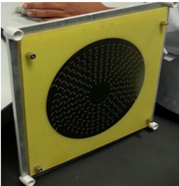
Figure 5: The slots on the surface of Air Gap RLSA prototype
