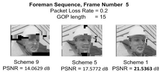
Figure 10: Comparison in Video frame quality of Foreman sequence using Scheme 1, Scheme 5 and Scheme 9
