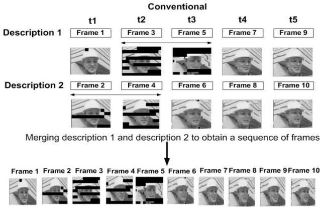
Figure 7: Illustration of a typical loss scenario of a GOP using a conventional scheme with Packet Loss Rate of 0.2.
