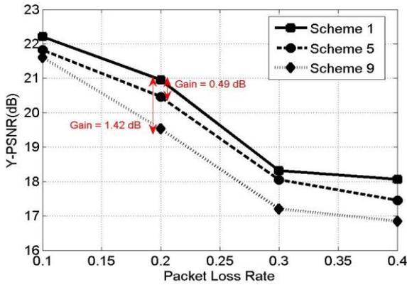
Figure 13: Graph of Y-PSNR against Packet Loss Rate with GOP length = 15 using MDC and the Composite channel model for the Foreman sequence
