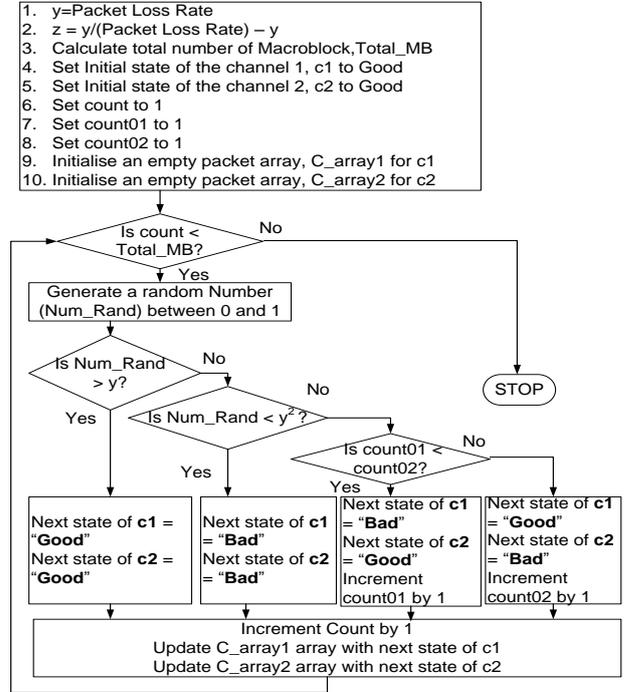
Figure 3: Flowchart illustrating the composite channel algorithm
