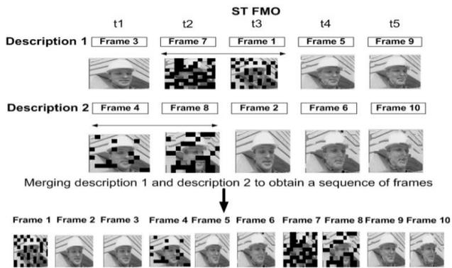
Figure 8: Illustration of a typical loss scenario of a GOP using ST-FMO with MDC with Packet Loss Rate of 0.2.
