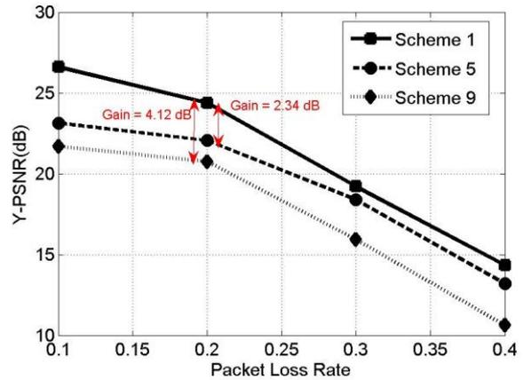
Figure 11: Graph of Y-PSNR against Packet Loss Rate with GOP length = 15 using MDC and Gilbert Elliot channel model for the Akiyo sequence
