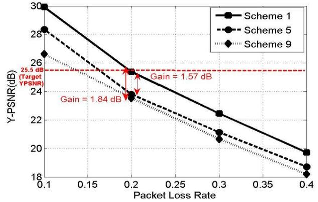
Figure 15: Graph of Y-PSNR against Packet Loss Rate with GOP length = 15 using MDC and the Composite channel model for the Akiyo sequence
