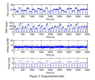
In this work, Polyethersulfone (PES) material with approximately 80-100kda pore size and the surface area is about  $0.35 \text{ m}^2$  membrane is used in the filtration system.
