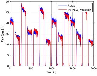
Figure 8: Permeate flux traning result
